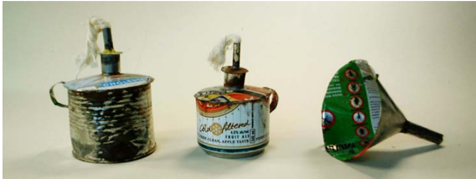
Figure 5. Kerosene lamps (and a filling funnel) fabricated from discarded food and drinks cans.
