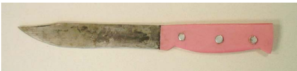
Figure 1. The knife handle is made from the plastic of an old bucket; the blade from a car panel
